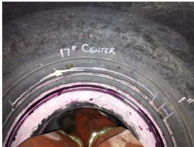
Figure 2: 17" Crack on Main Valve Seat
